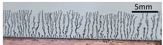
Figure 1: Dendrites formed on the cathode during an electrodeposition sequence.
