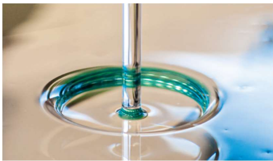
Figure : Circular hydraulic jump (silicone oil).
